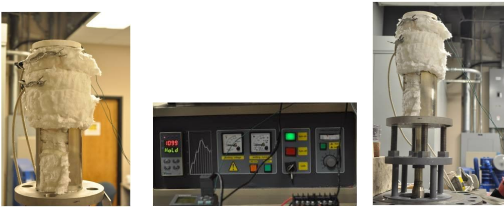
Figure 3.11 Thermal cycling experimental set up including furnace heater, temperature controller and furnace holder
