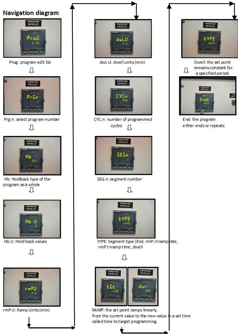
Figure 3.9 Flowchart of the basic operation of CM 1700 programmable furnace equipped with a 2404 control set point program
